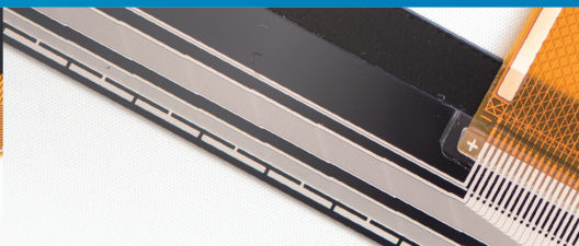
Laser etching production process for ultra-thin border
